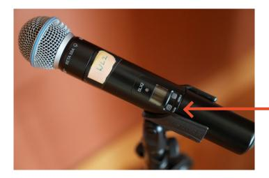
Power on the Microphone using the Power Button. If it is out of battery, you will need to locate a 9 volt battery from the Maintenance Room.\*
